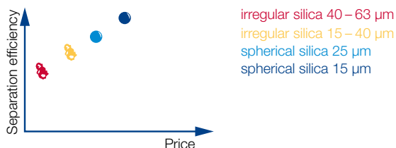
Comparison of separation efficiency and price of irregular versus spherical silica
