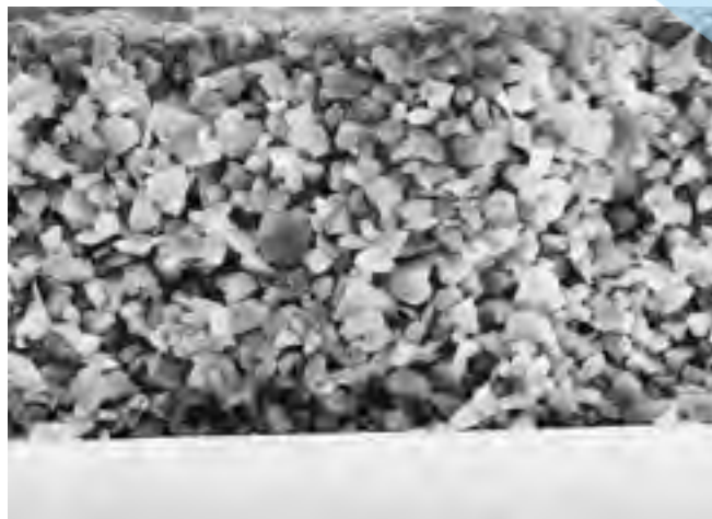
Electron microscope photograph of a cross section through a glass plate with silica layer (magnification × 500)
