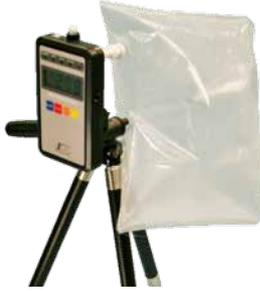
Collects samples into a sampling bag directly for air sampling in work environment.
