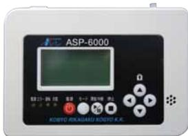
Designed to be used with gas detector tubes and sorbent tubes and to collect dust with a holder for collection and liquid with a impinger.
