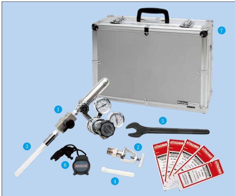
Impurities in breathing air for respiration can adversely affect human health. The kit is designed to measure these contaminants in SCBA, SCUBA and other pressurized breathing air cylinders, as well as directly from the outlet of an air compressor or purifier. The kit easily measures five components within minutes : carbon monoxide, carbon dioxide, oil mist, water vapor and oxygen by aerating the detector tube with an exclusive reducing valve from the breathing air source.
