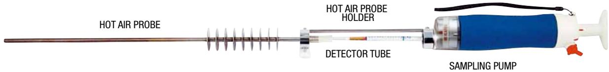
Remove the connector holder of the sampling pump and connect the hot air probe holder and the sampling pump. Break both ends of the detector tube and connect to the hot air probe. Open the screw knob and insert the detector tube into the hot air probe holder. Insert the detector tube into the rubber tube connector of the sampling pump, then close the screw knob.
